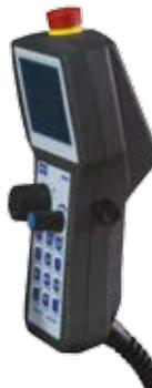
It is equipped with the basic safety functions for a remote device such as the emergency button and the "dead man" button to ensure maximum safety for the operator. The 3.5" graphic display allows to visualize functional pages realized through the HTML language and structured as Web pages, thanks to the Web Server and client (APACHI) present in the terminal.
